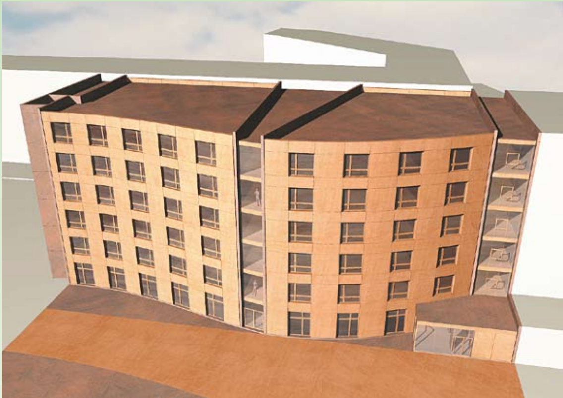
Figure 4: Six-storey residential care home in solid timber construction in Berlin-Lichtenberg (scheduled for realisation in 2008). Source: Kerbl Architekten, www.kerbl-architekten.de
