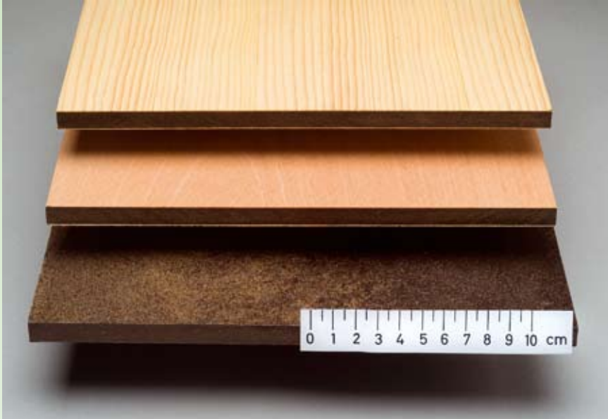
Figure 3: Surfaces and workability of ARBOFORM® construction boards.
