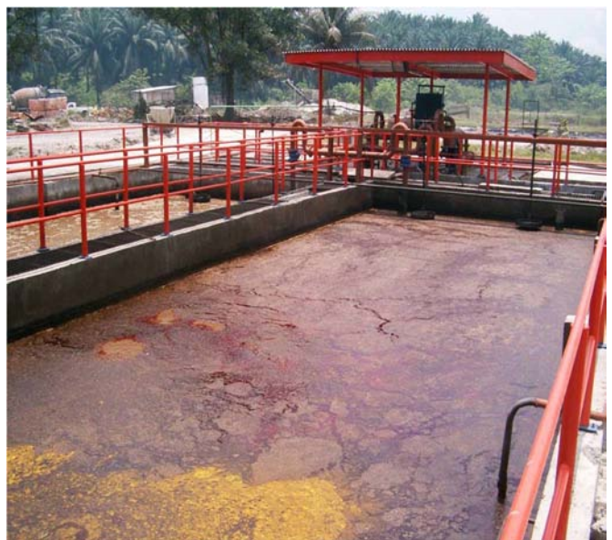
Picture 4: Effluent arising from the extraction of palm oil is temporarily stored in a cooling basin. Photograph: IFEU
