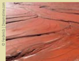
The other side of the (aluminium) coin: red mud tailings – unused residue from the aluminium production.
