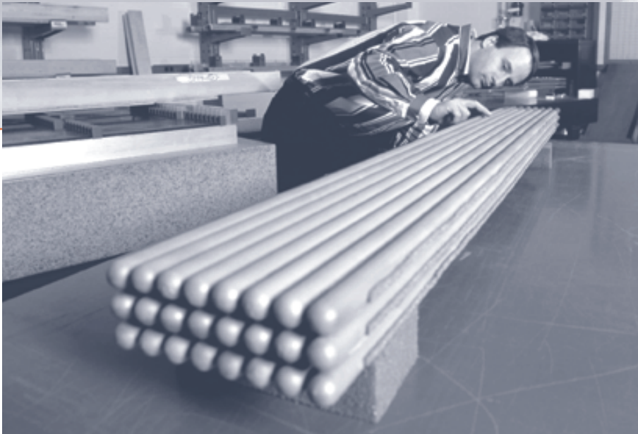
The Solid Oxide Fuel Cell consists of many of these ceramic tubes. Each of these tubes will deliver 200 Watt.
